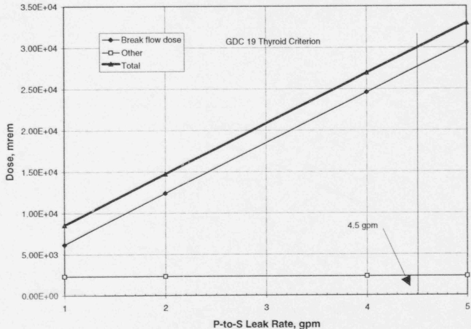
Control Room Dose vs Leak Rate
