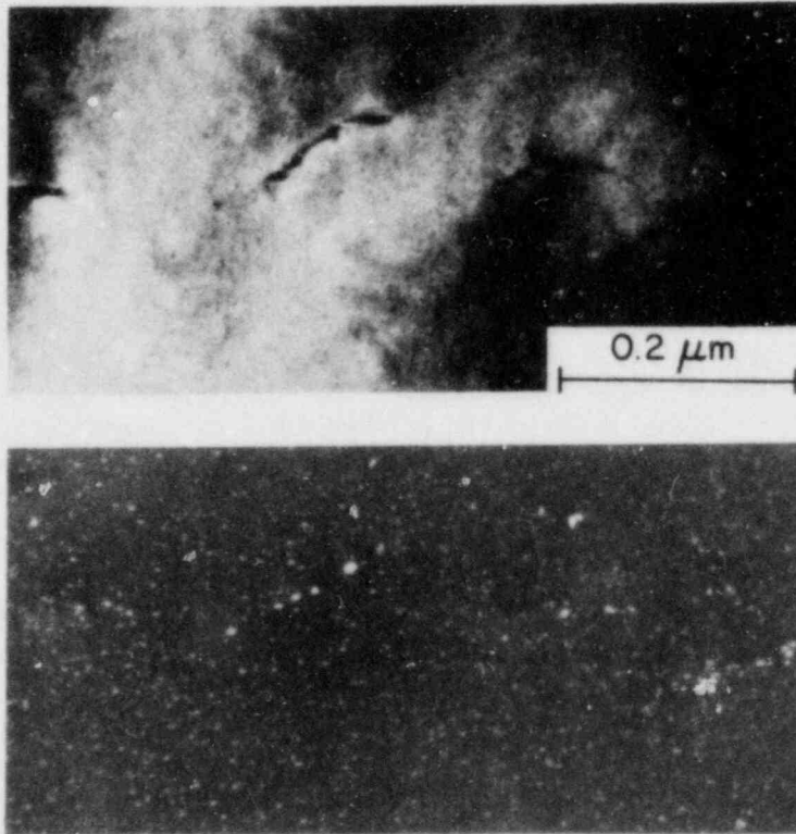
Fig. 4.6. Bright- and Dark-Field Images of Precipitates in CF-8 Stainless Steel (Heat 278) Aged for 70,000 h at 300°C.
