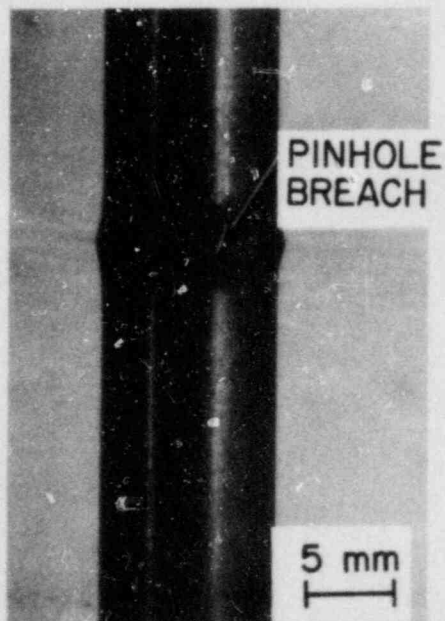
Fig. 3.29. Pinhole Leak Indication in H. B. Robinson Specimen 217A4E at the 247^\circ Orientation. Helium pressure 6.9 MPa.
