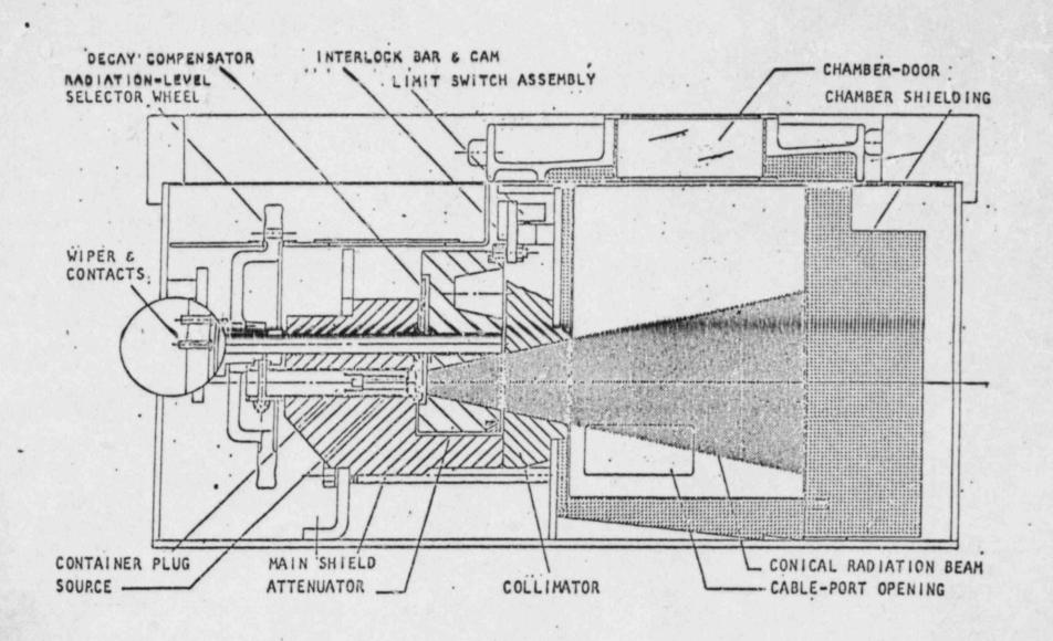
Source Housing for the CDV-794 Model 2 Calibrator
