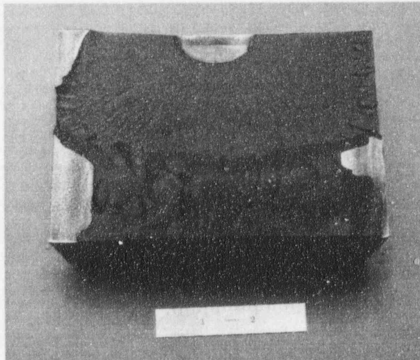
Figure 2.13 Fracture surface of finite-length flaw specimen CF-4
