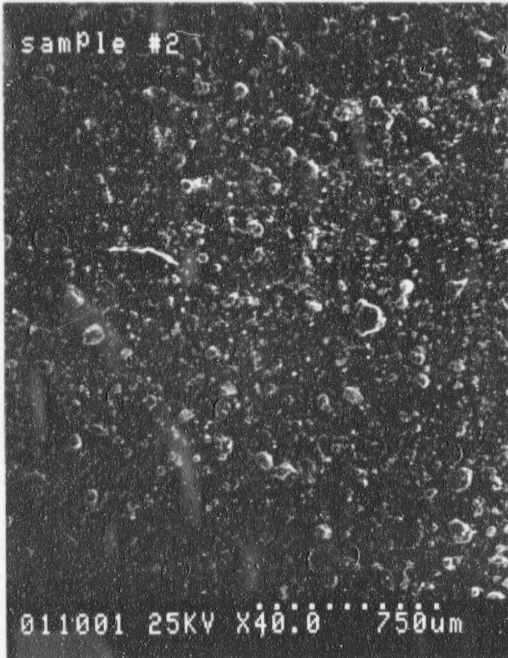
Figure E-7 SEM of Sludge A Collected After Circulating in Test Loop (750 \mu\text{m} magnification)
