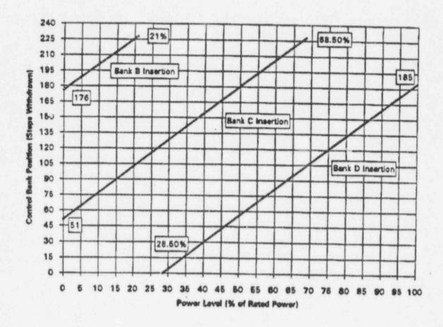
Note: The "fully withdrawn" parking position range can be used without violating this Figure.
