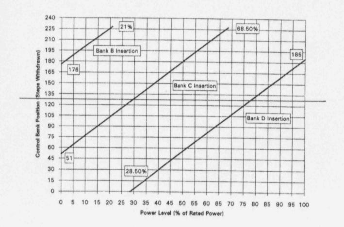
Note: The "fully withdrawn" parking position range can be used without violating this Figure.
