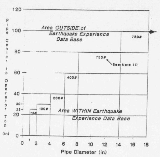
(1) Approximate Maximum Operator Weights Given for Various Ranges of Pipe Diameter
