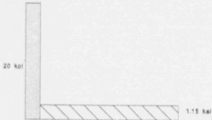
CLAD STRESS DISTRIBUTION
