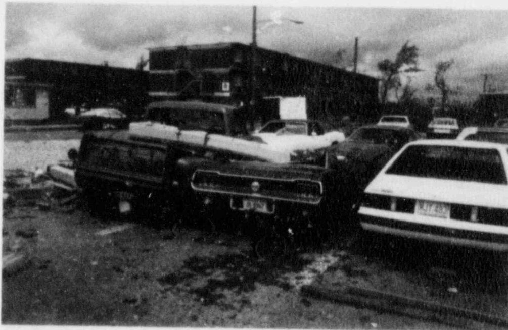
FIGURE 9. CONCRETE MASONRY BOND BEAM MISSILE (missile traveled from the base lawyer's office northeastward approximately 200 feet before striking the vehicles).
