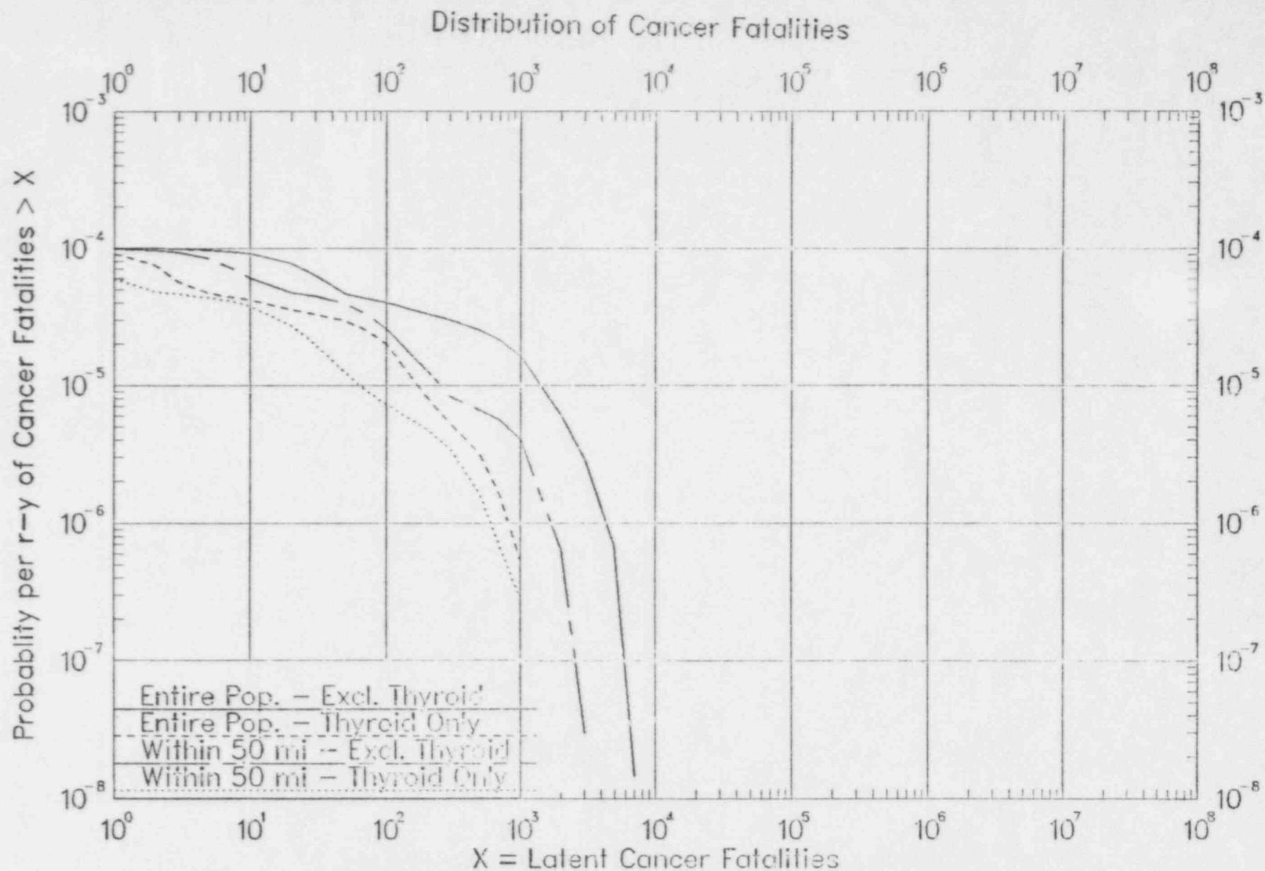
Figure 5.7 Probability distributions of cancer fatalities. (See Section 5.9.4.5(7) for a discussion of uncertainties in risk estimate (50 miles = 80 km). Also see a footnote in section entitled "Dose and Health Impacts of Atmospheric Releases" for help in interpreting this figure.)
