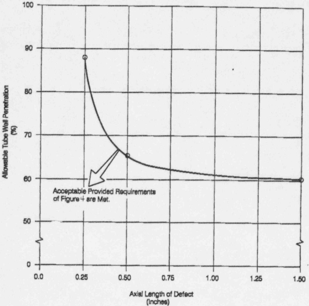
Figure 4. Maximum Allowable Penetration Versus Arc Length For 34.1 % Maximum Allowable Area of (From Reference 8.2)
