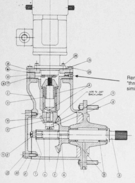
Remove oil line and verify "through" hole using wire or similar object.
