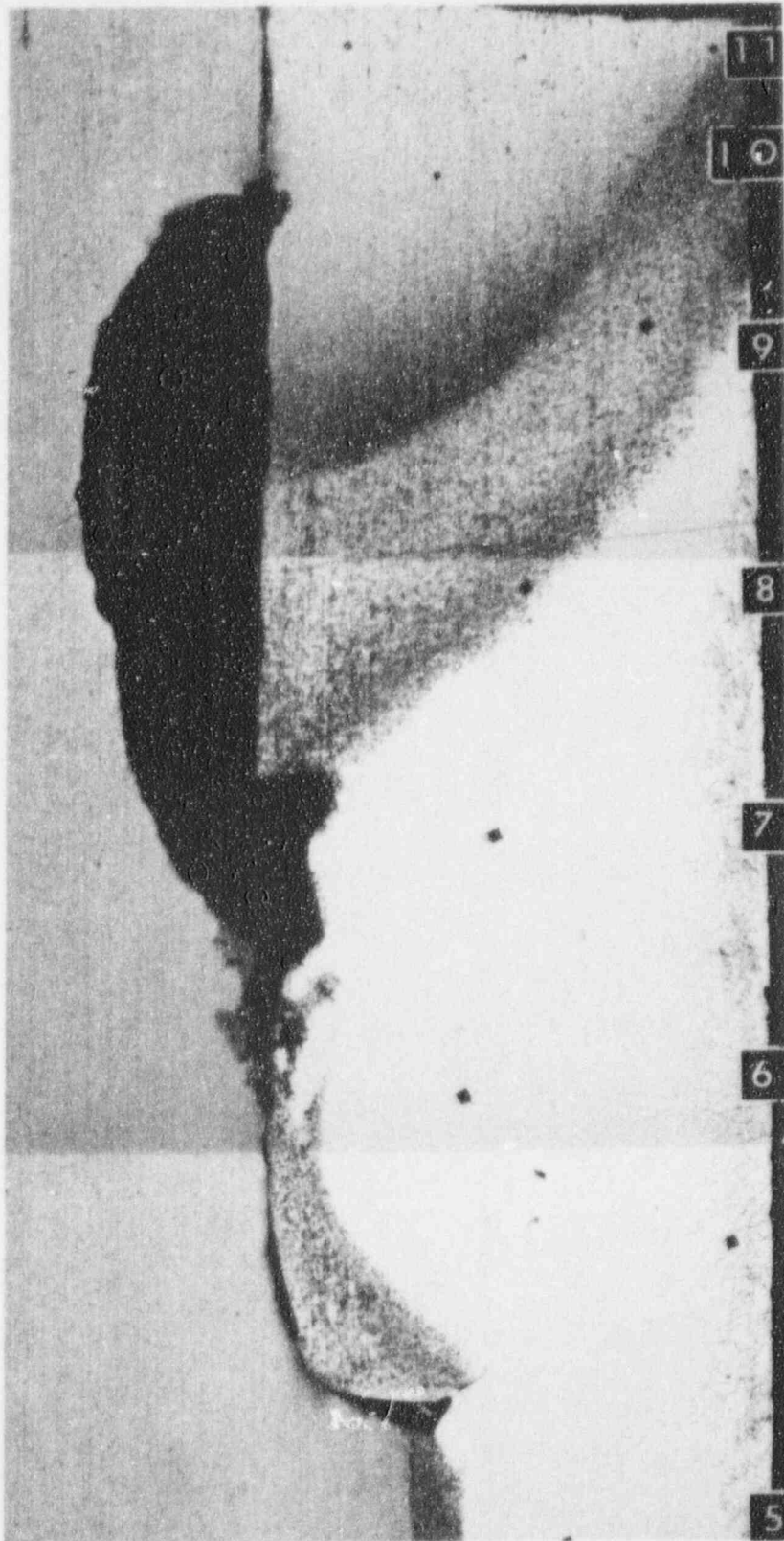
FIGURE 5-2. PHOTOMICROGRAPHS OF THE ROD CROSS SECTIONED SHOWING THE WELD AND MICROHARDNESS LOCATIONS.
