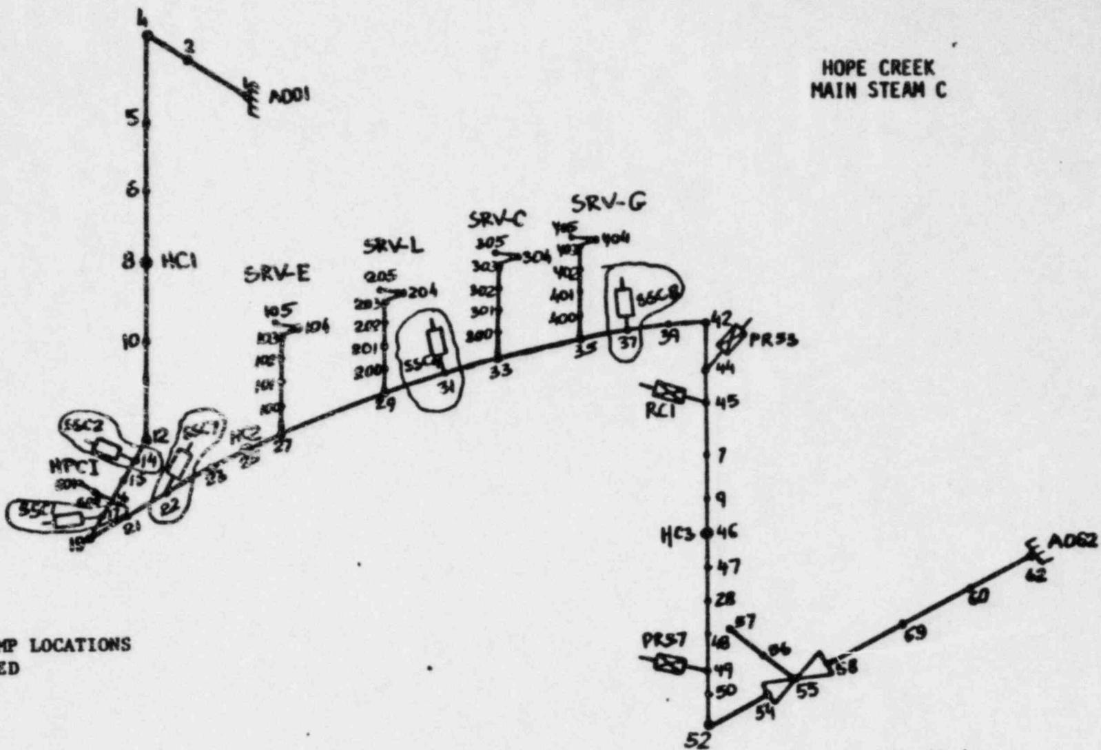
FIGURE A-1 NODE DIAGRAM FOR MAIN STEAM LINE C
