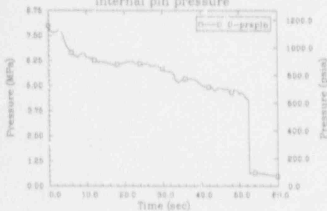
SEABROOK 100%DBA 5 GWD/MTU PIN--PF 2.0 (TRAC) internal pin pressure
