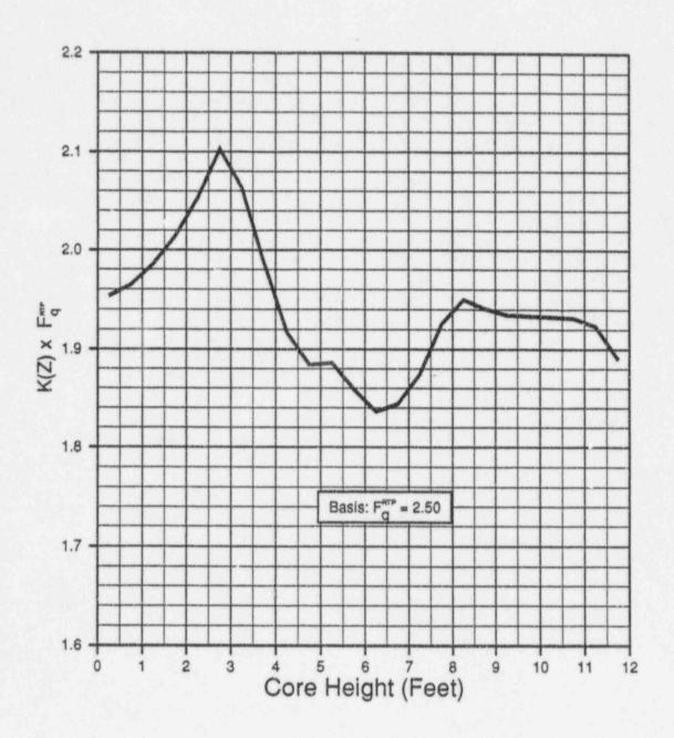
F<sub>Q</sub> (Z) Limit As A Function of Core Height for Operation with Fixed Incore Detector System Alarm Inoperable and Cycle Average Burnup 8.0 to 14.0 GWD/Mtu
