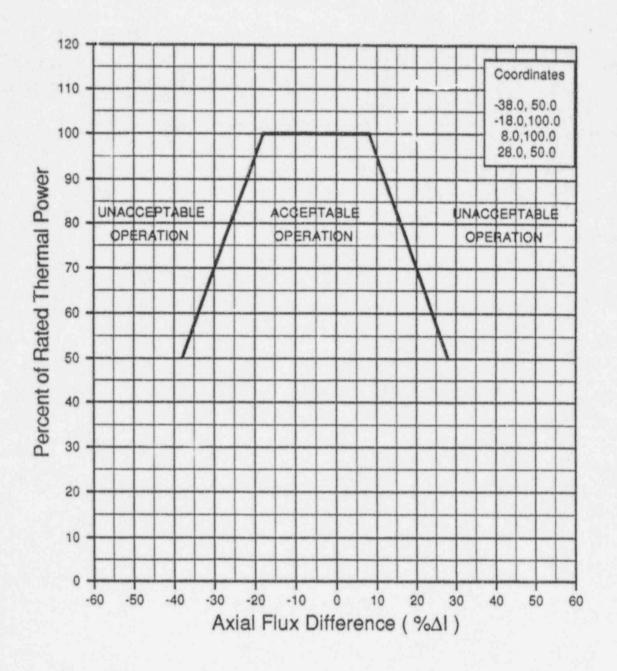
Axial Flux Difference Limits as a Function of Rated Thermal Power for Operation With Fixed Incore Detector System Alarm OPERABLE
