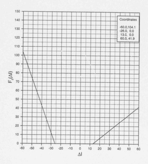
Overpower  $\Delta T$  Trip  $F_2(\Delta I)$ Axial Flux Imbalance Penalty Function
