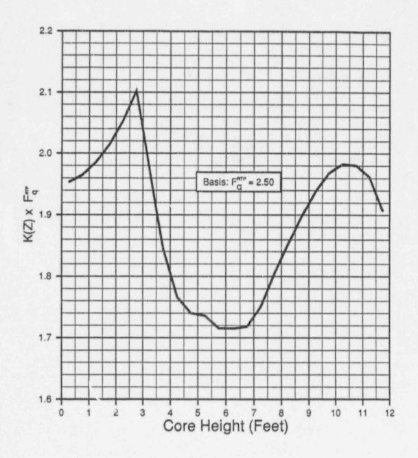
F<sub>g</sub> (Z) Limit As A Function of Core Height for Operation with Fixed Incore Detector System Alarm Inoperable and Cycle Average Burnup > 14.0 GWD/Mtu
