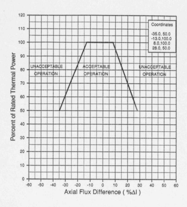
Axial Flux Difference Limits as a Function of Rated Thermal Power for Operation With Fixed Incore Detector System Alarm Inoperable
