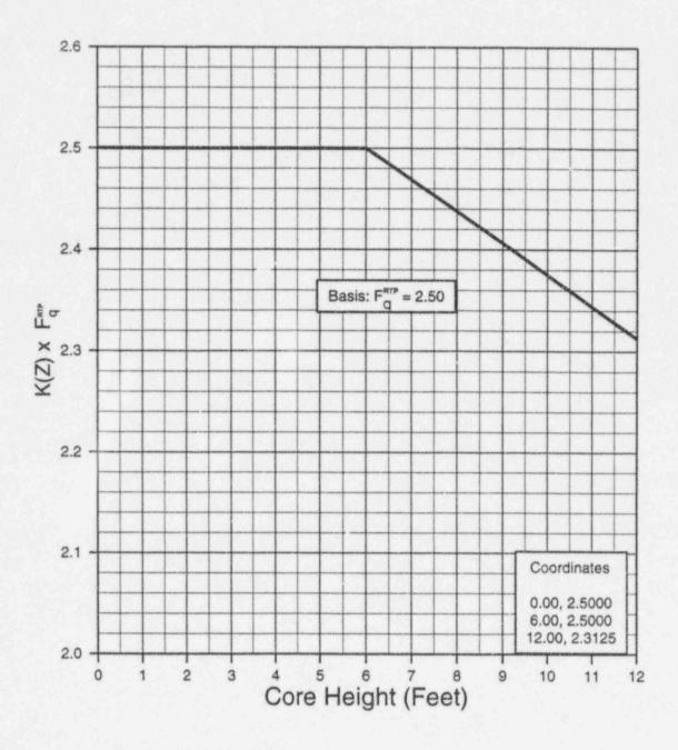
F<sub>g</sub> (Z) Limit As A Function of Core Height for Operation with Fixed Incore Detector System Alarm OPERABLE
