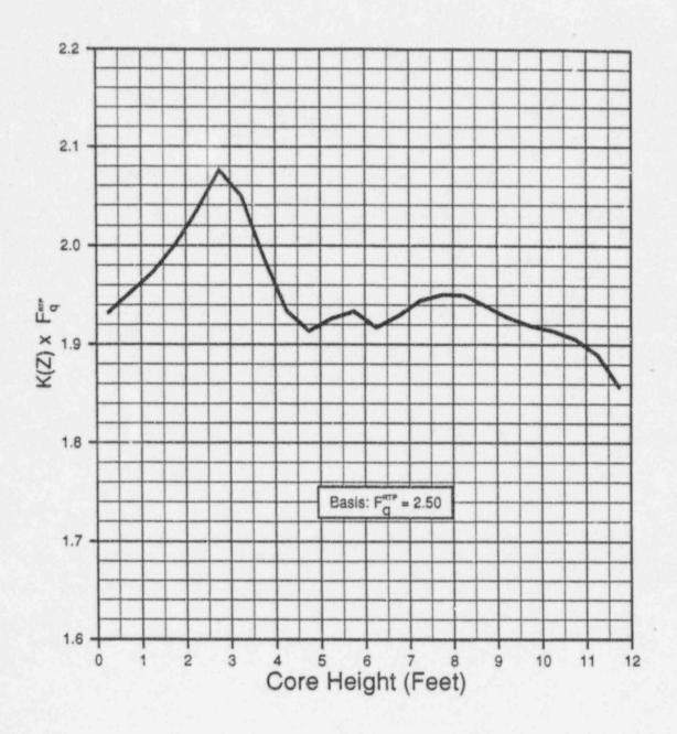
F<sub>g</sub> (Z) Limit As A Function of Core Height for Operation with Fixed Incore Detector System Alarm Inoperable and Cycle Average Burnup < 8.0 GWD/Mtu
