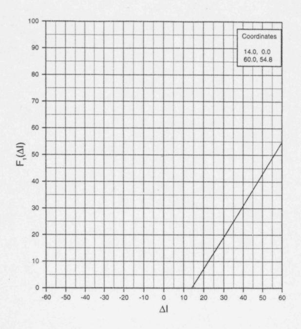
Overtemperature  $\Delta T$  Trip F,( $\Delta I$ ) Axial Flux Imbalance Penalty Function
