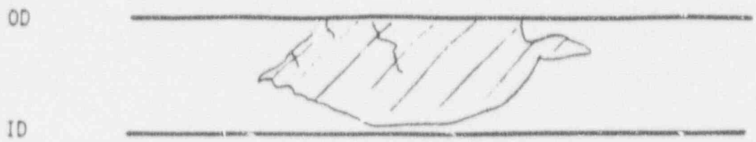
Sketch of Burst Crack
