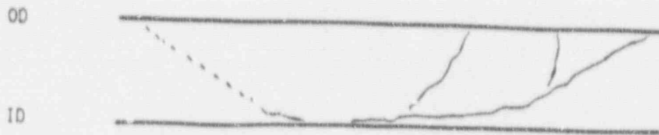
Sketch of Burst Crack
