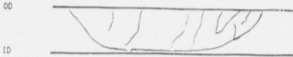
Sketch of Burst Crack
