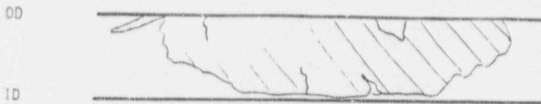
Sketch of Burst Crack
