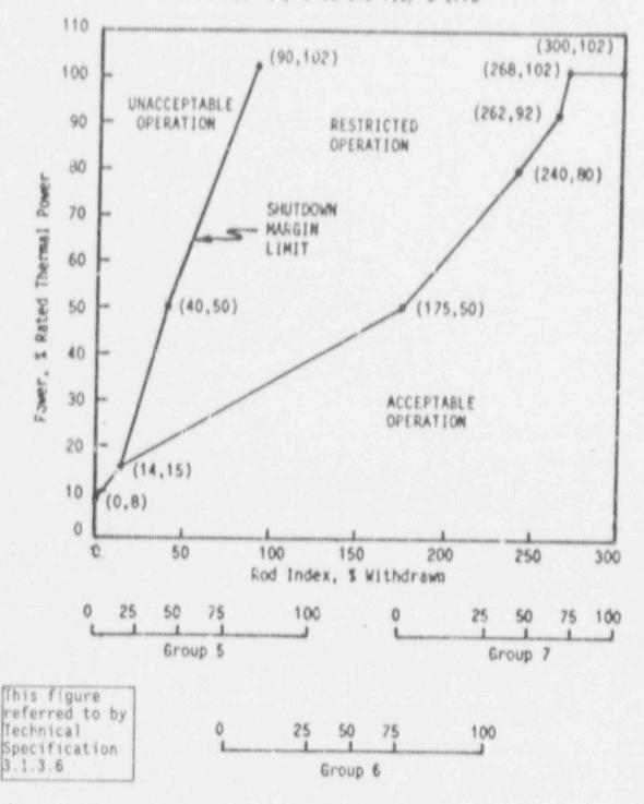
Note 1: A rod group overlap of 25  $\pm$  5% between sequential withdrawn groups 5 and 6, and 6 and 7 shall be maintained.
