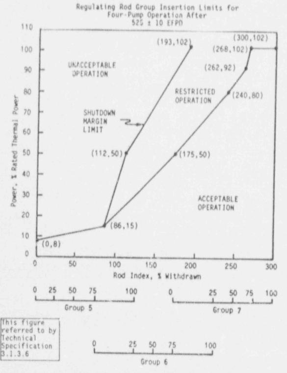
Note 1: A rod group overlap of 25 ± 5% between sequential withdrawn groups 5 and 6, and 6 and 7 shall be maintained.
