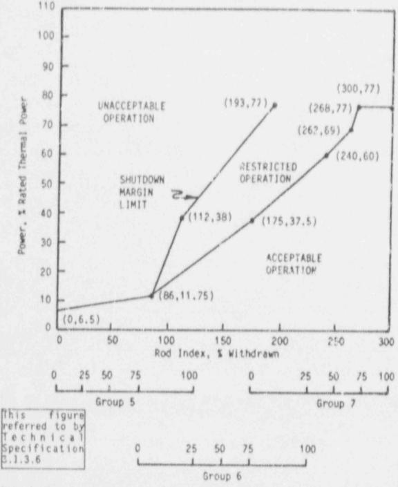
Note 1: A rod group overlap of 25 ± 5% between sequential withdrawn groups 5 and 6, and 6 and 7 shall be maintained.
