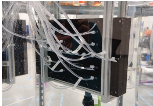
Fluid dynamics tests Room-temperature water 40% geometric scale
