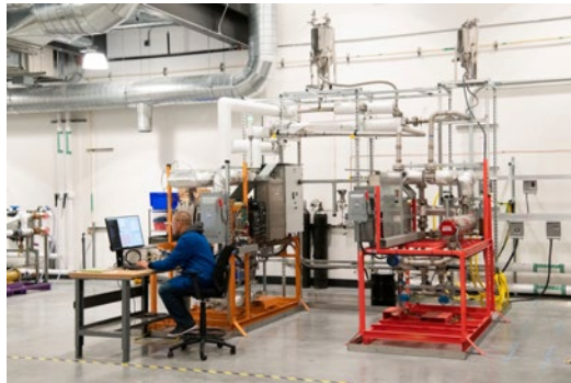
Heat transfer tests Heat transfer oil (72°C) Reduced geometric scale
