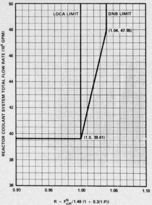
PENALTIES OF 0.1% FOR UNDETECTED FEEDWATER VENTURI FOULING AND MEASUREMENT UNCERTAINTIES OF 2.1% FOR FLOW AND 4.0% FOR INCORE MEASUREMENT OF  $F_{\Delta H}^N$  ARE INCLUDED IN THIS FIGURE.
