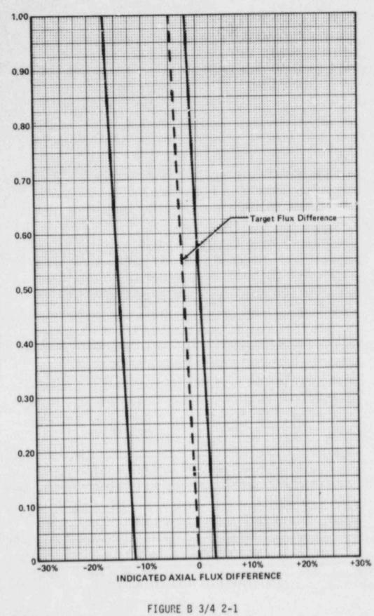
TYPICAL INDICATED AXIAL FLUX DIFFERENCE VERSUS THERMAL POWER
