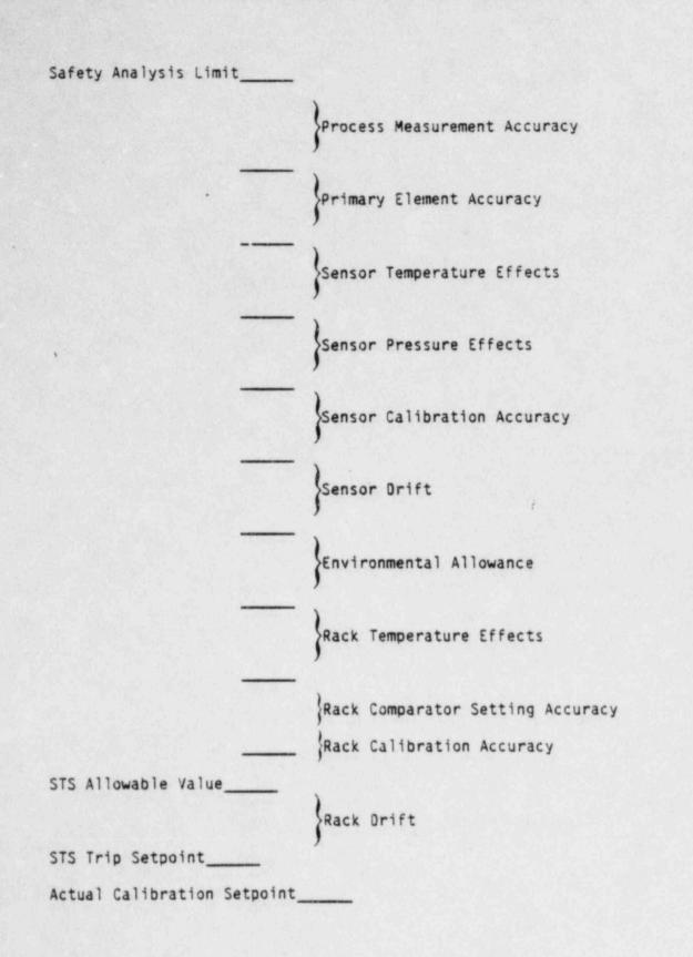
Figure 4-1 NUREG-0452 Rev. 4 Setpoint Error Breakdown
