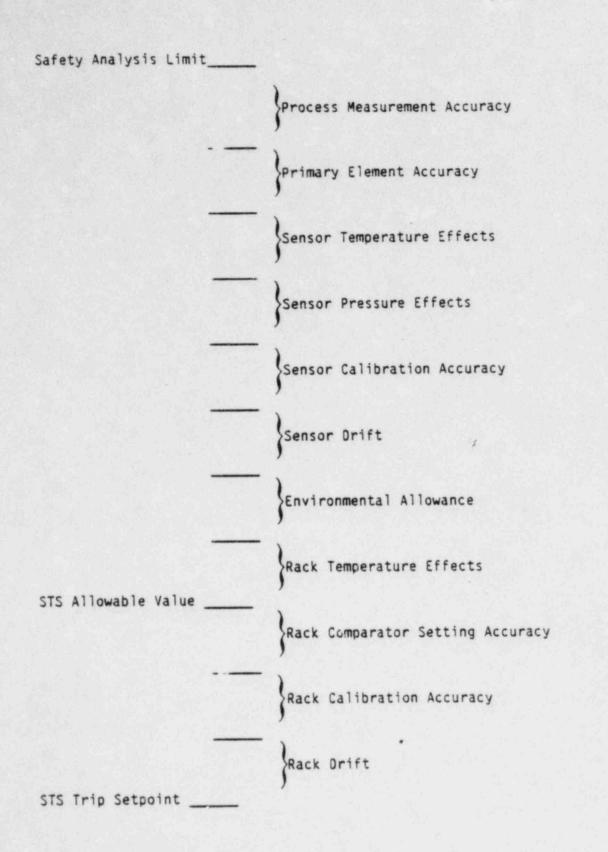
Figure 4-2 Westinghouse STS Setpoint Error Breakdown
