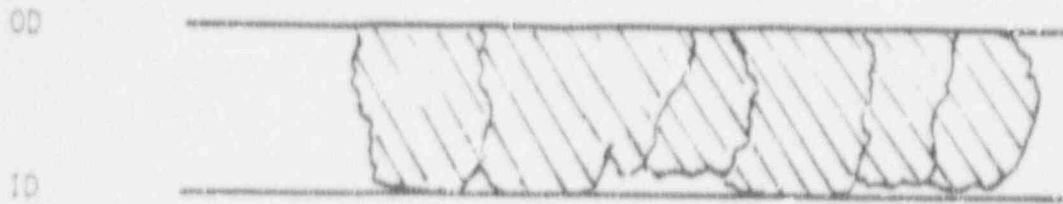
Sketch of Burst Crack
