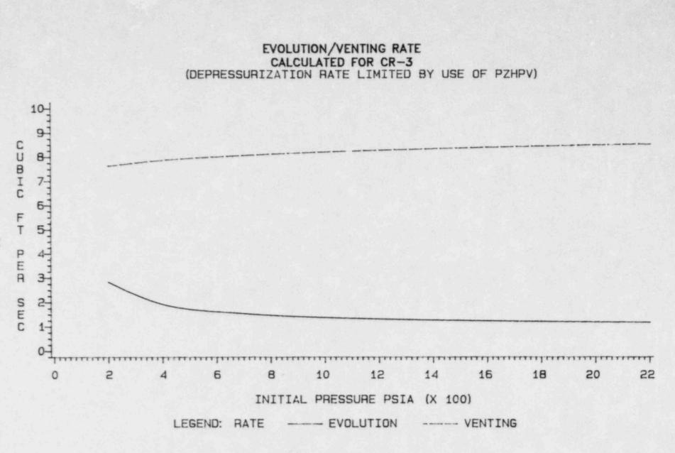
NOTE1: VENTING RATE FOR HYDROGEN USING 2 HLHPV NOTE2: EVOLUTION RATE FOR HYDROGEN FROM RV HEAD AND RCS
