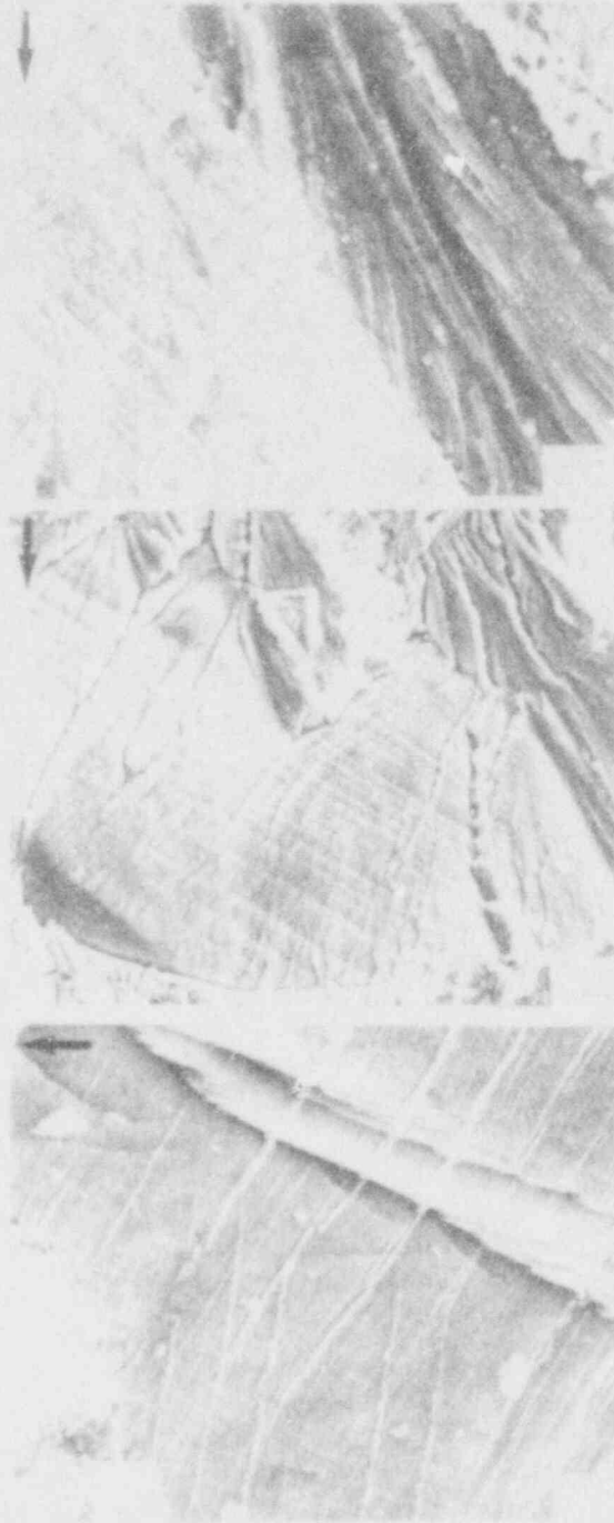
Figure 2.11 Fractographic features of environmentally-assisted fatigue crack growth in SA 351-CF8A cast stainless steel. \Delta K \sim 20 \text{ MPa}\sqrt{\text{m}} . Test temperature was 288^\circ\text{C} . The linear features are slip steps which have been "decorated" with oxide.
