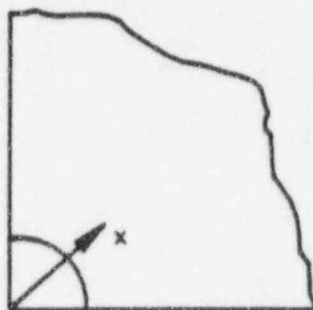
FUN 10 - QUARTER-CIRCULAR CRACK IN QUARTER-SPACE
