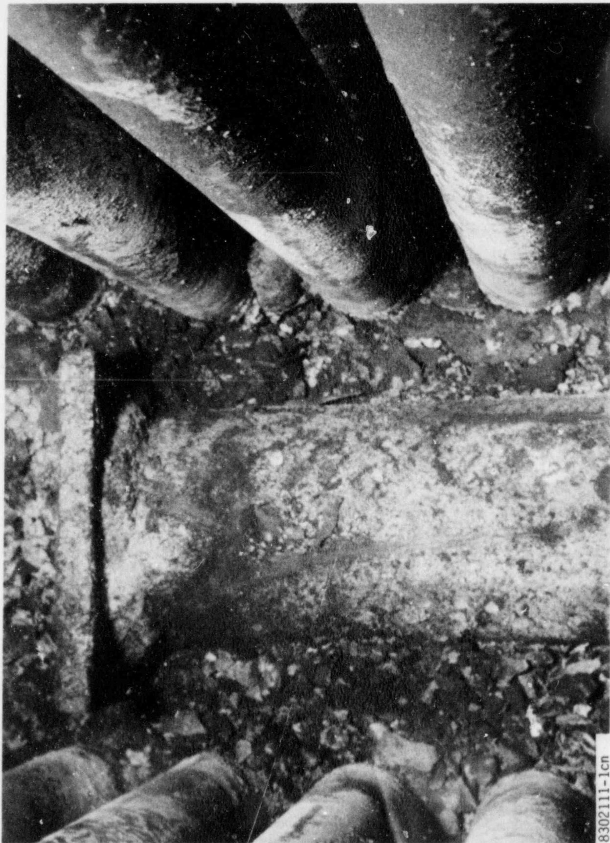
FIGURE 11. Close-Up View of Tube Sheet/Blowdown Pipe Region Around Center of Generator
