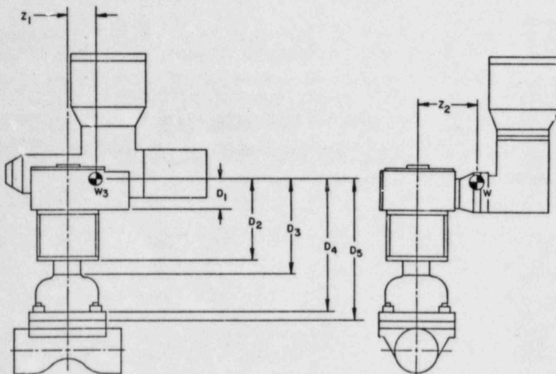
DESIGN DATA FOR A 2 IN. POWER OPERATED DIAPHRAGM VALVE
