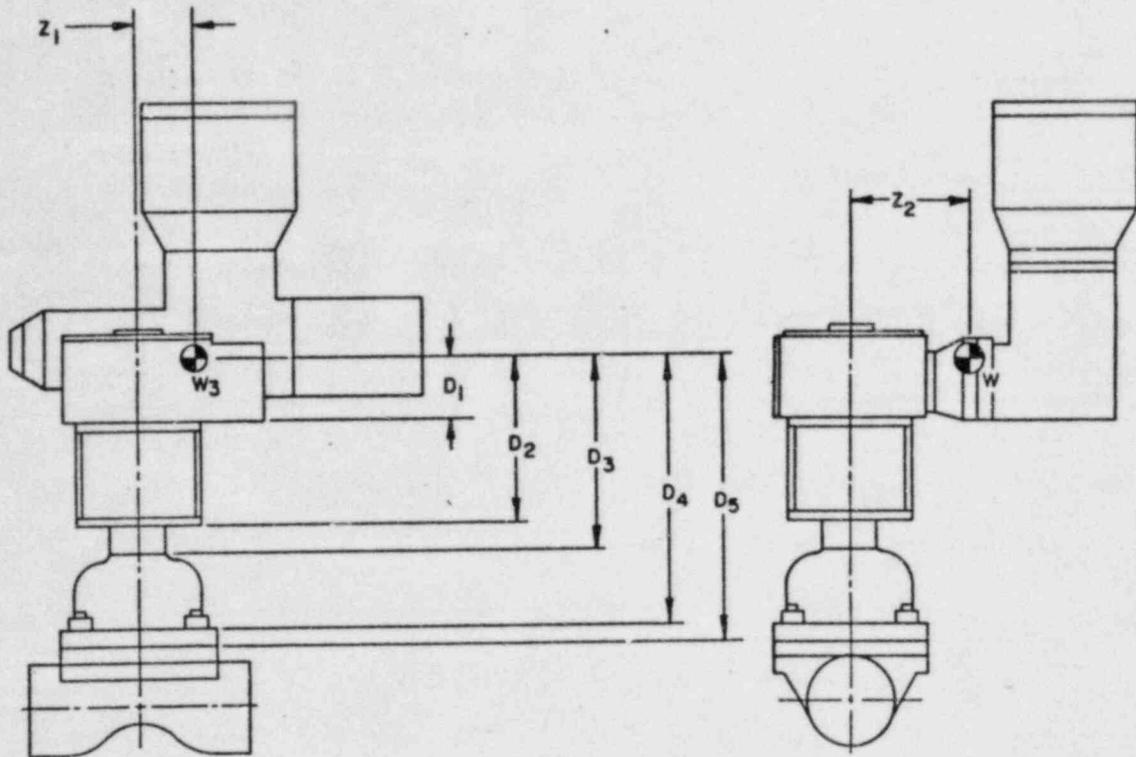
DESIGN DATA FOR A 4 IN. POWER OPERATED DIAPHRAGM VALVE
