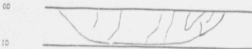
Sketch of Burst Crack
