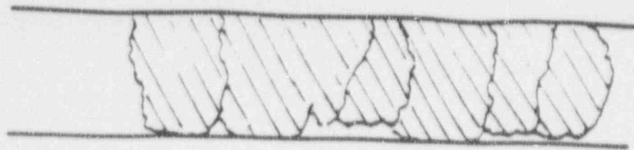
Sketch of Burst Crack
