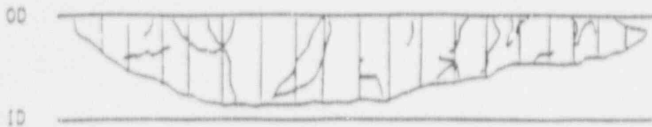
Sketch of Burst Crack
