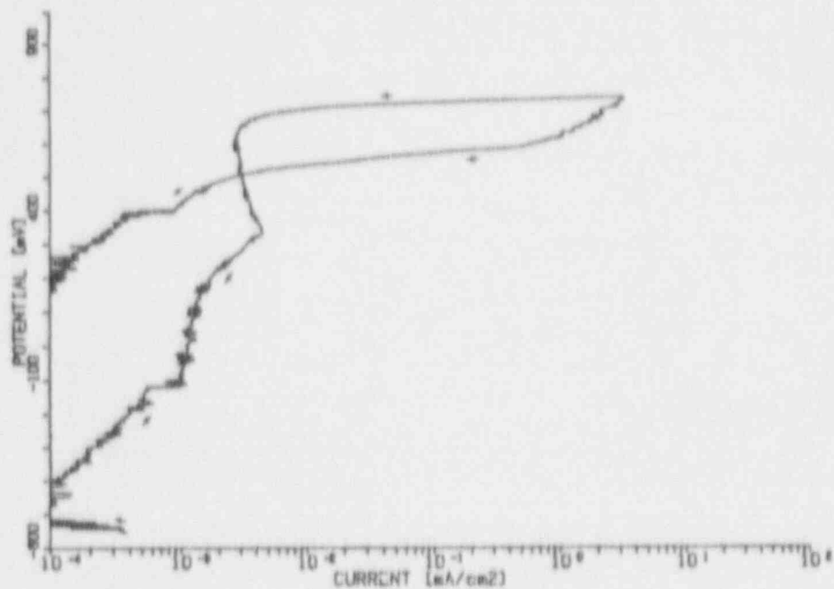
Figure D11. Potentiodynamic Polarization Curve For Alloy 825 In Solution No. 11 At 90°C.
