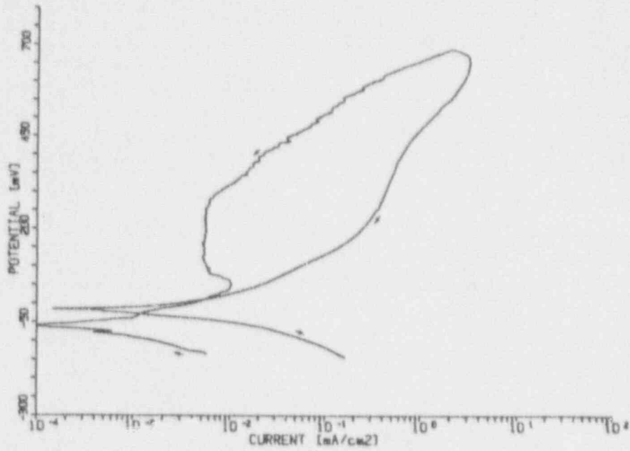
Figure B29. Potentiodynamic Polarization Curve For Alloy CDA 715 In Solution No. 29 At 50°C.
