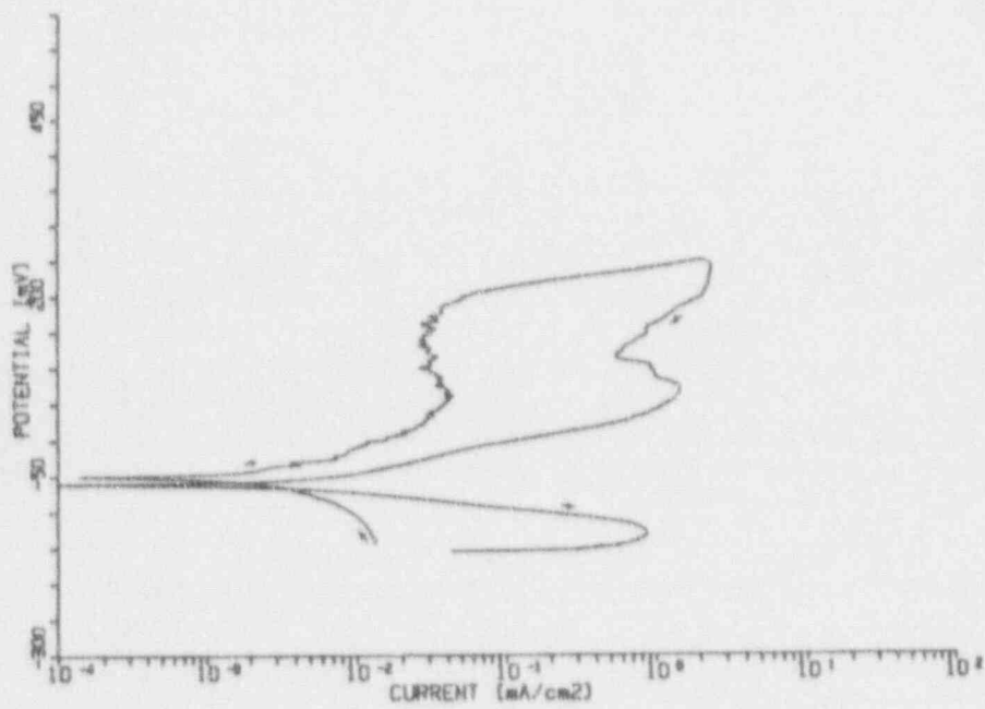
Figure B28. Potentiodynamic Polarisation Curve For Alloy CDA 715 In Solution No. 28 At 90°C.
