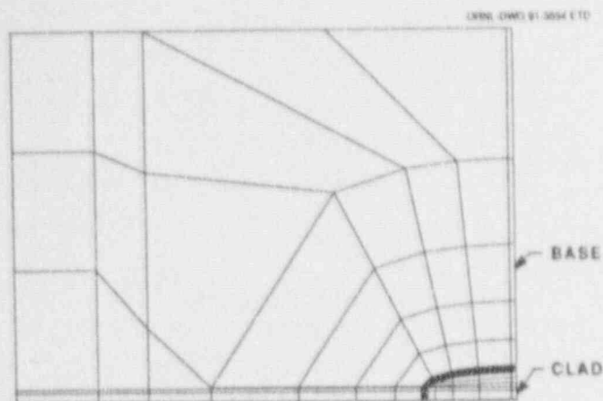
Figure 7.3 Close-up view of crack-tip region of clad cylinder
