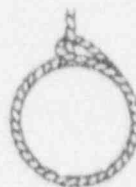
Bad-Because of cutting action of eye splice on running line
