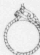
Bad-Bolt on running line can work loose
