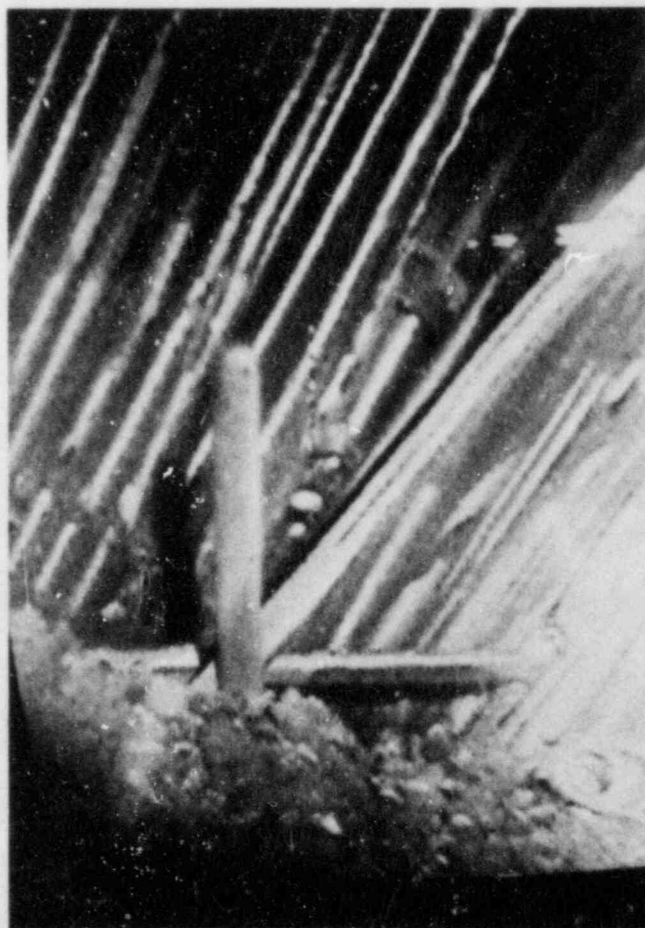
The photograph shows the upper part of the nuclear core of the TMI-2 reactor, with portions of fuel elements (the white strips) lying on the rubble bed and, in one case, protruding from it.
