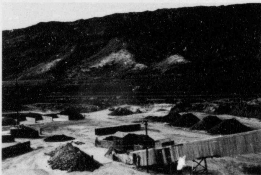
Uranium ore is segregated and stored until processing at the Atlas Uranium Mill in Moab, Utah.
