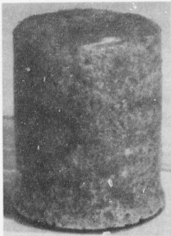
Figure 7. ASTM control waste-form specimen after being immersed for 66 days in medium containing nitrifying bacteria.
