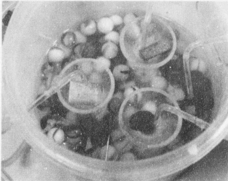
Figure 28. Waste form placement in misting chamber.
