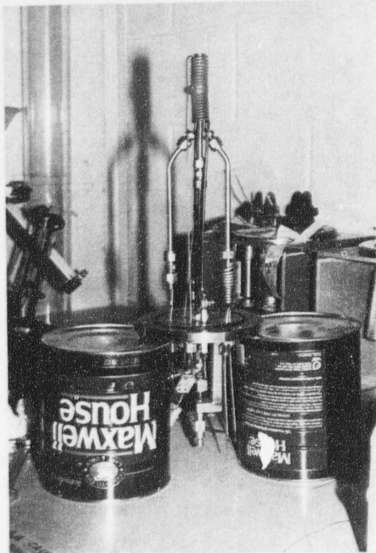
Figure 2.8 Reactor Chamber Mounted on Pump Flange
