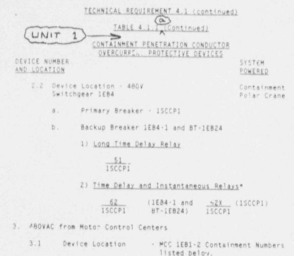
Primary and Backup - Both primary and backup breakers Breakers - Both primary and backup breakers have identical trip ratings and are in the same MCC Compt. These breakers are General Electric type THED or THFK with thermalmagnetic trip elements.
