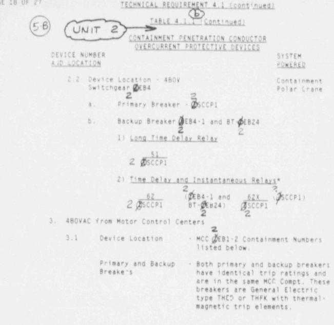
Associated circuit breaker(s) shown in parantheses; e.g. ØEB4-1 and BT-ØEB24 are backup breakers for ØSCCP1.
