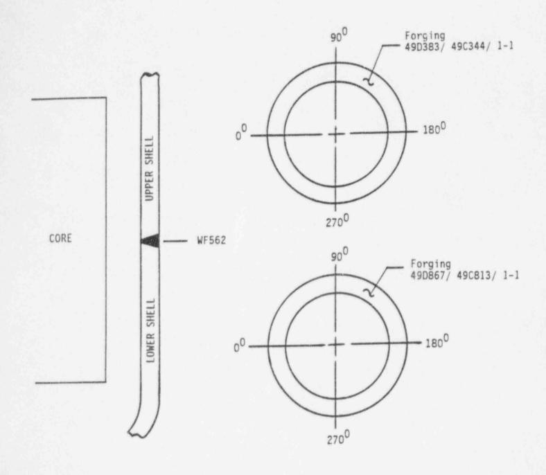
Figure 1 Identification and Location of Beltline Region Material for the Braidwood Unit 1 Reactor Vessel<sup>[6]</sup>
