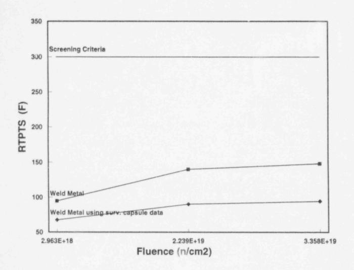
Figure 2 RT<sub>PTS</sub> versus Fluence Curves for Braidwood Unit 1 Limiting Material - Weld Metal
