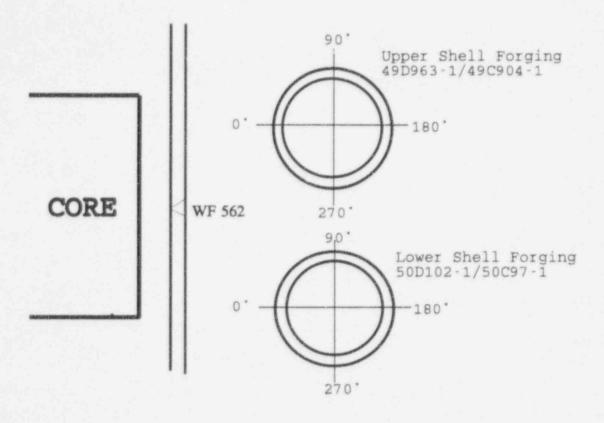
Figure 1 Identification and Location of Beltline Region Material for the Braidwood Unit 2
