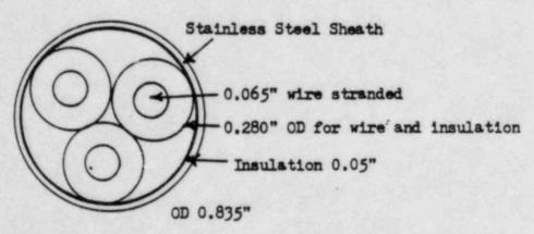
All dimensions are nominal, with the OD of the non-stainless steel sheath being 0.630 inch.
