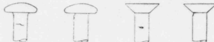
FIGURE 2. Transverse discontinuities in the head or shank.
