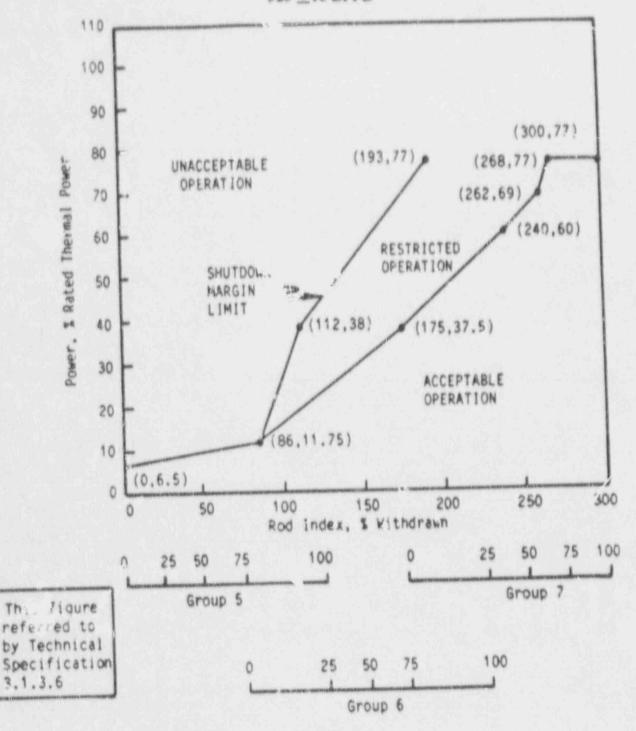
Note 1: A rod group overlap of 25 ± 5% between sequential withdrawn groups 5 and 6, and 6 and 7 shall be maintained.
