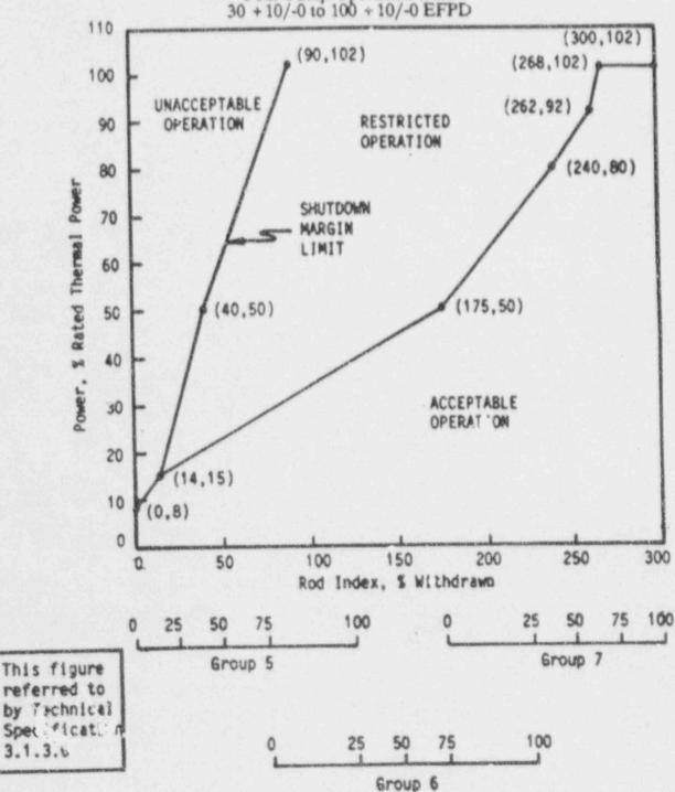
Note !: A rod group overlap of 25 ± 5% between sequential withdrawn groups 5 and 6, and 6 and 7 shall be maintained.
