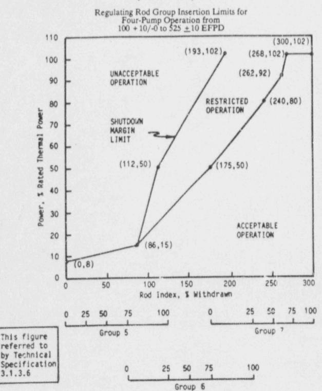
Note 1: A rod group overlap of 25 ± 5% between sequential withdrawn groups 5 and 5, and 6 and 7 shall be maintained.
