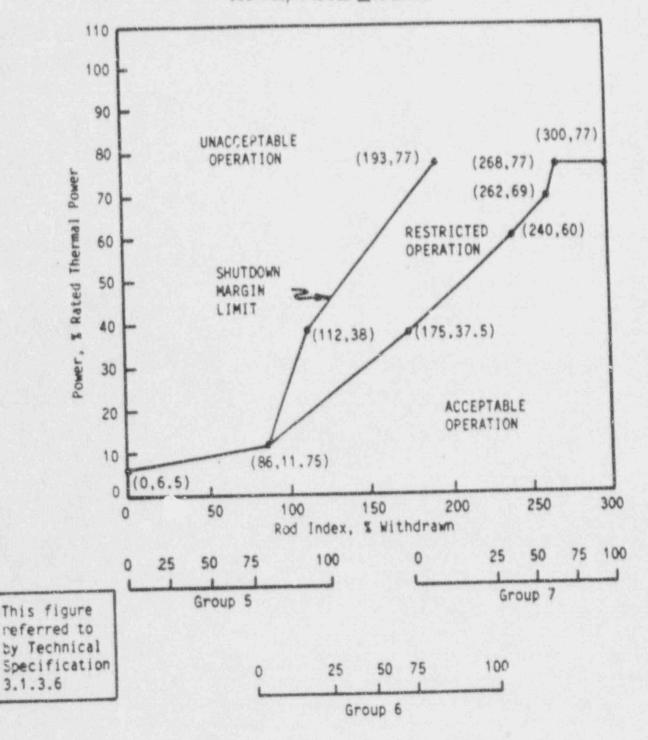
A rod group overlap of 25 + 5% between sequential withdrawn groups 5 Note 1: and 6, and 6 and 7 shall be maintained.
