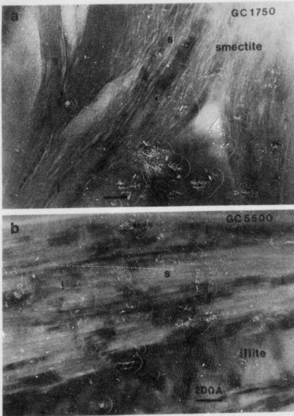
Figure 16. TEM lattice-fringe images of samples from Gulf Coast sediments at two different depths, (a) 1750 m and (b) 5500 m showing changes in smectite and illite layer proportions: (a) At 1750 m depth, smectite is dominant over illite. Smectite layers are characteristically very irregular and imperfect. Small packets of illite (i) occur within smectite. (b) At 5500 m depth, illite is the dominant mineral. The layers are relatively regular and well crystallized but show some imperfections along grain boundaries (packet boundaries) with mottled contrast feature. Smectite (s) is rare and shows very little contrast because it is easily damaged by the electron beam relative to illite. (photos from Lee et al., 1984a)
