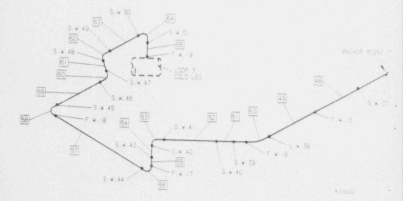
"F.W." means field welds. (these are SMAW) "S.W." means shop welds. (these are GTAW) "he numbers in the squares identify the materials. (see the ID column of table 3-1)
