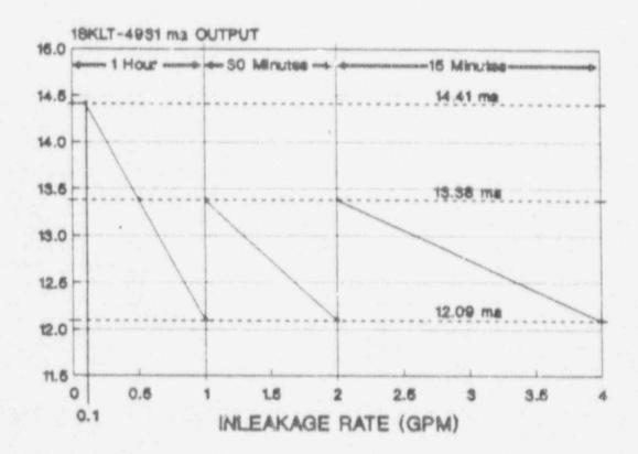
Sump should be pumped down at or above the intersection of the current rate and MA output.
