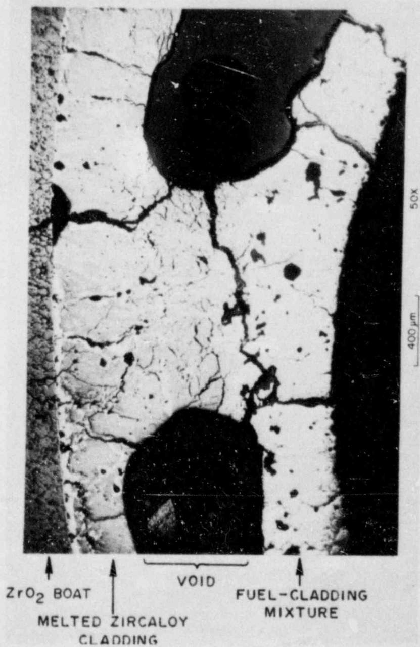
Fig. 25. View of midlength region (cut 6) of fuel specimen from test HI-3, showing extensive melting and interaction of Zircaloy cladding and UO 2 fuel. With the exception of small chips, no intact UO 2 was found in this region.
