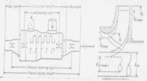
Hydrostatic bearings offer significant reduction in boiler feed pump size and cost. Their lead-carrying capacity is maintained by an externally pressurized fluid. Hence, fluid film separates shart from bearing even at zero speed.
