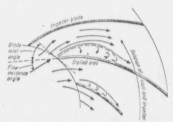
Stalling occurs when the incidence angle—difference between flow angle and pump-impeller or diffuser vane inlet angle—increases above a specific critical value. Stalled area, which eventually washes out, respirms as rotation continues.
