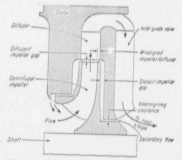
Vibration, cavitation, and instability can generally be traced to one of several possible locations in a centrifugal pump stage. For example, wearing-ring clearance might be excessive or perhaps the impeller/diffuser is out of alignment
