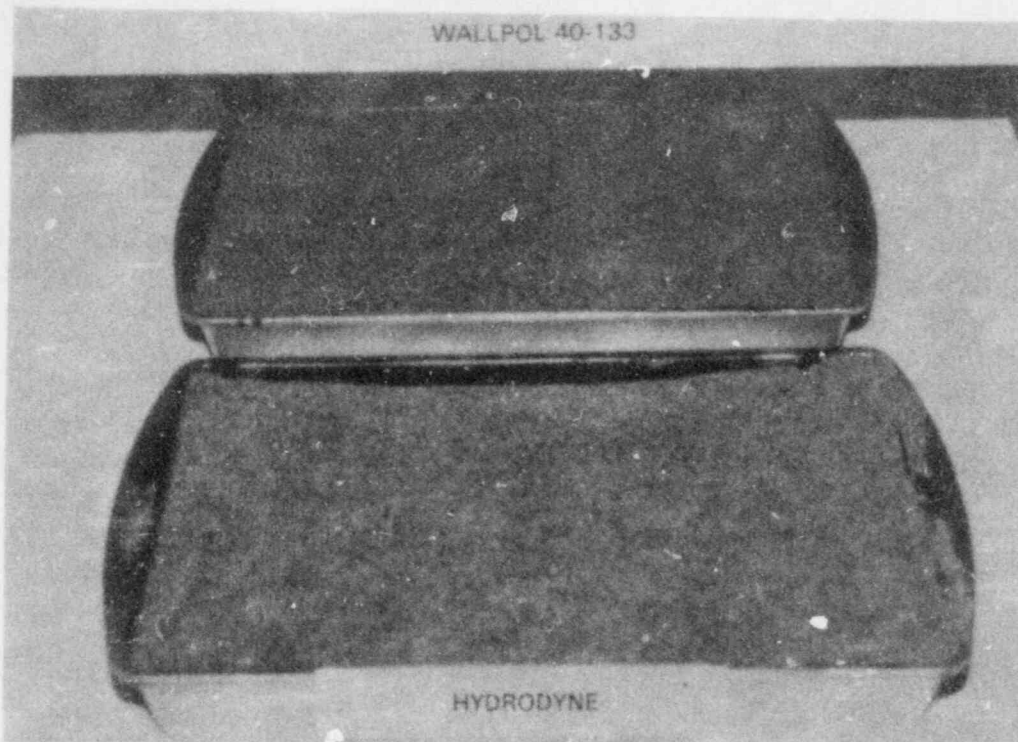
FIGURE 6. Sample Pans Stabilized with Wallpol 40-133 (more durable) and Hydrodyne C (less durable)
