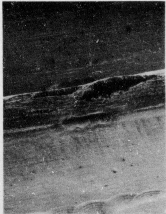
Figure B-16. Apparent sheath blowout along Thermocouple TE-REB-E1 in the embedded region (50X).
