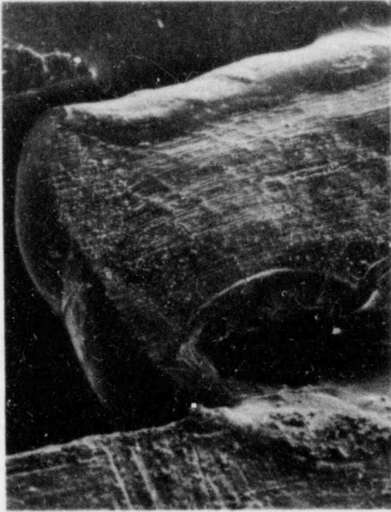
Figure B-9. Sheath burn-through at embedded junction of Thermocouple TE-REB-E1 (200X).
