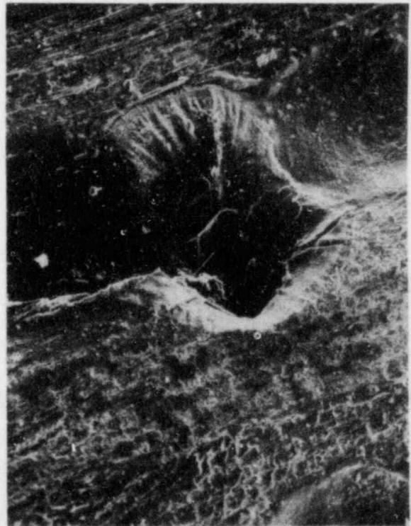
Figure B-12. Sheath burn-through at a laser weld along Thermocouple TE-REB-E2 (200X).
