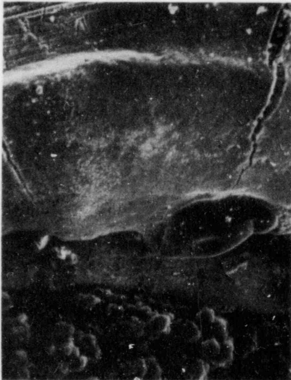
Figure B-10. Sheath burn-through at embedded junction of Thermocouple TE-REB-E1 (1000X).
