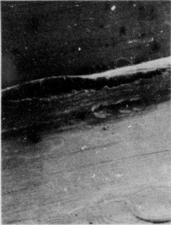
Figure B-13. Apparent sheath blowout along Thermocouple TE-REB-E1 in the embedded region (50X).
