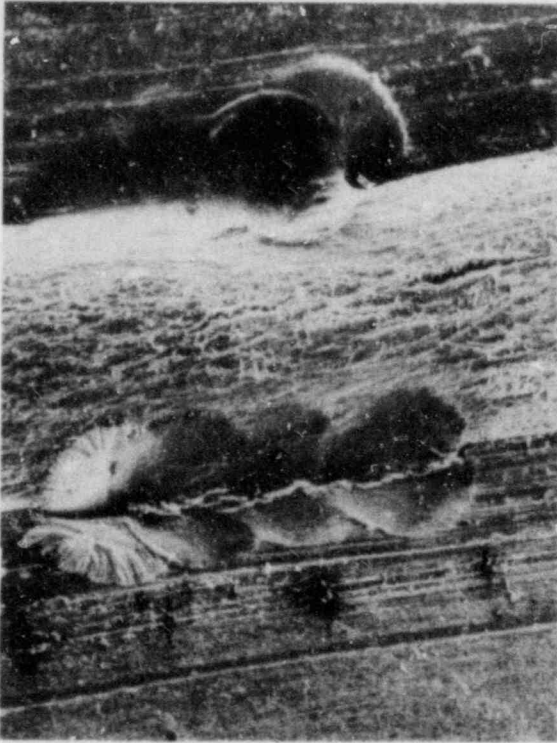
Figure B-6. Cracks in sheath of Thermocouple TE-REB-E2 near a laser weld (100X).
