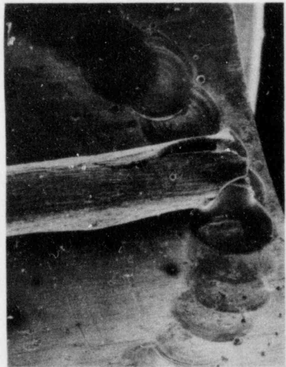
Figure B-19. Burn-through of Thermocouple TE-REB-E1 sheath at cladding insert laser weld (50X).
