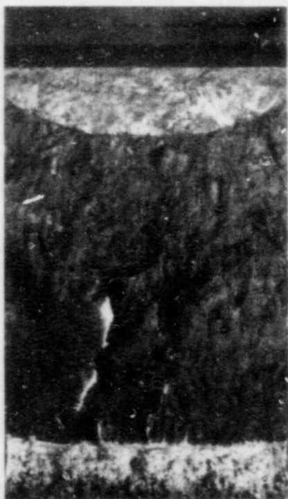
Fig. 12a. Macro photographs of the specimens tested in the axial orientation for three temperatures, 232°C, 288°C and 338°C (450°F, 550°F and 640°F). The crack front tended to have a somewhat irregular profile for this orientation.
