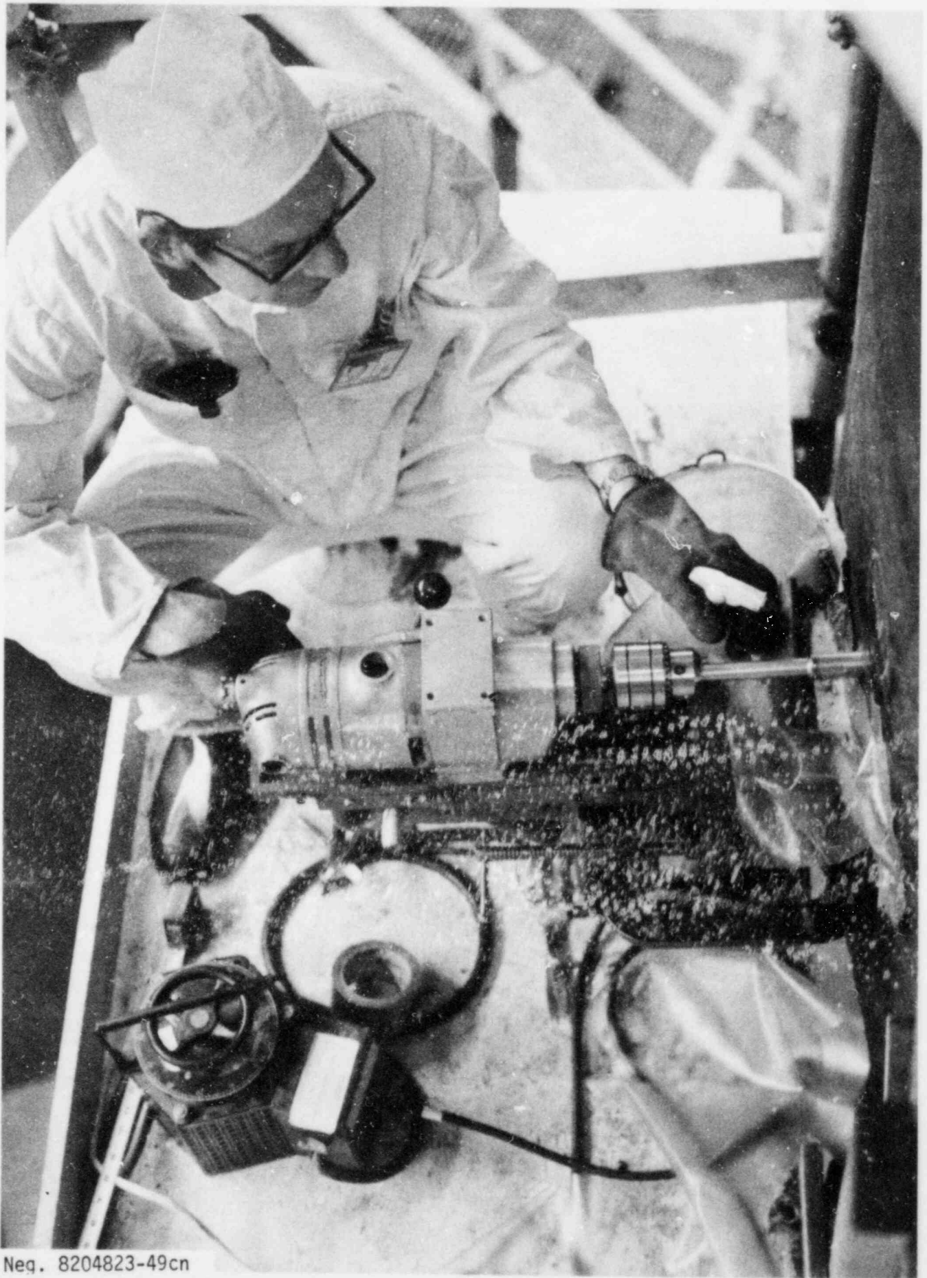
FIGURE 60. Drilling Core Sample from Channel Head
