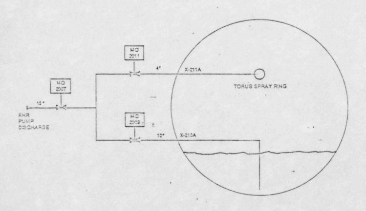
Figure 2. Torus Spray and Recirculation Lines.
